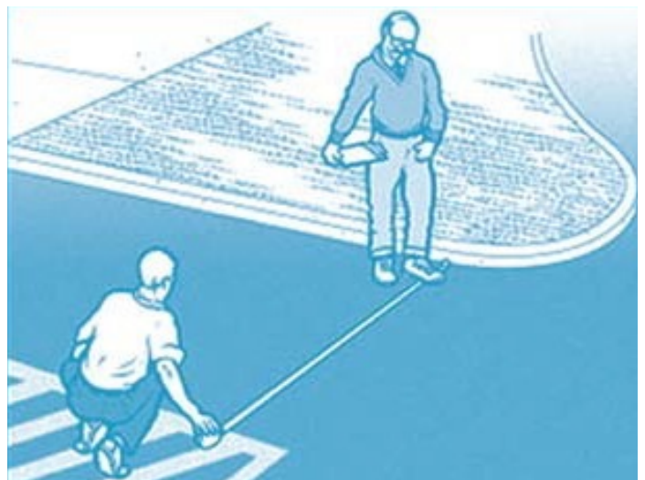
Image 4: Using a tape measure to measure the width of a parking space.
